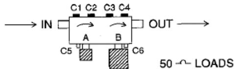
2. Adjust capacitors C1 through C4 for minimum insertion loss at the centre frequency.
