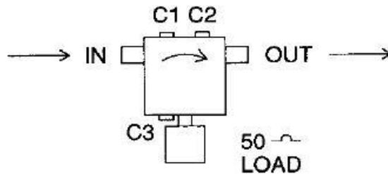
3. Reverse connections to the isolator in/out ports and adjust capacitor C3 to obtain typical isolation at  $F_0$  (=35 dB).
