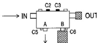
11. Adjust C2 and C3 for maximum isolation at the load port A. (This may require several minor back and forth adjustment for C2 and C3.). At this point, we are matching the two stages.
